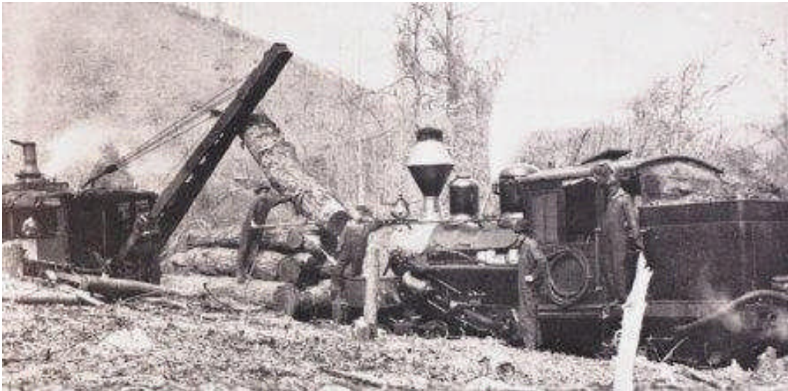
28-ton, two-truck Climax number 3 with log loader. #3 was built in 1899 and the loader was American Log Loader, model E. The location is unknown.
